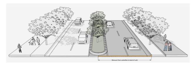
Label and dimension the existing and future curb and gutter from the centerline for each road on the site plan.
