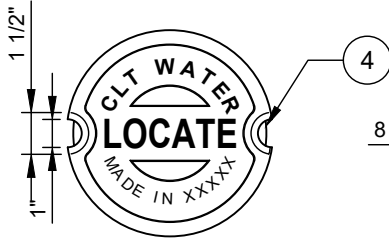
TRACER WIRE TERMINAL POINT COVER TOP - VIEW
