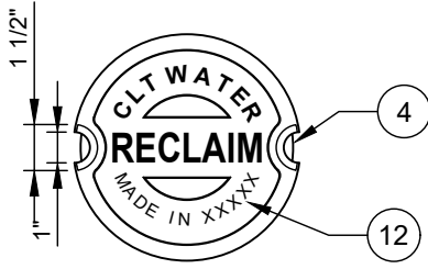
RECLAIMED WATER - TOP VIEW
