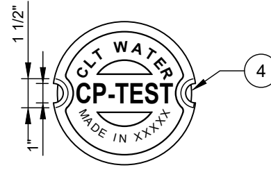
CATHODIC PROTECTION COVER TOP - VIEW
