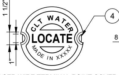
TRACER WIRE TERMINAL POINT COVER TOP - VIEW
