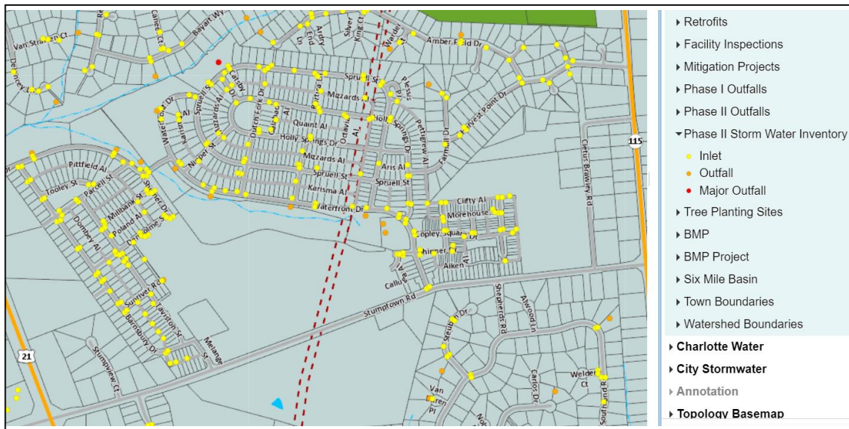
Figure 8: Screen Shot from Cityworks of Storm Drain Inlets, Outlets, and Receiving Streams The storm sewer system map is updated daily by Mecklenburg County’s GIS Department in order to capture inlets and outlets added by new development. This is completed as part of their
