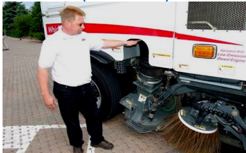
Figure 18. Vacuum Truck (NCSU-BAE)
