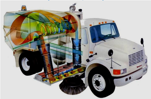
Figure 17. Regenerative Air Cleaner (TYMCO, Inc.)
