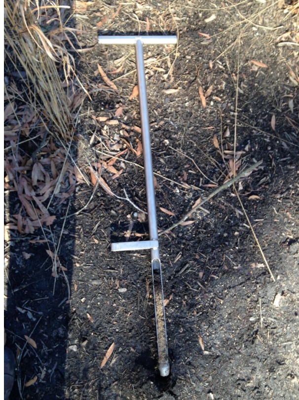
Figure 5: Soil Probe Showing a Profile of Bioretention Cell Media
