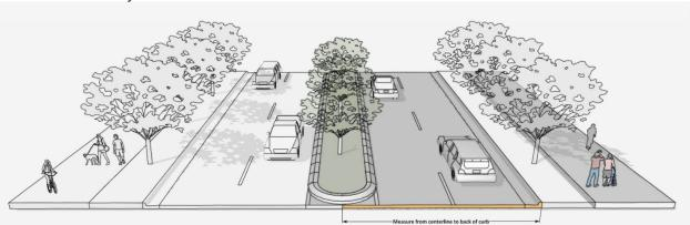
Label and dimension the curb and gutter from the centerline for each road on the site plan.
