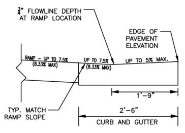
2'-6" CURB AND GUTTER RAMP DETAIL
