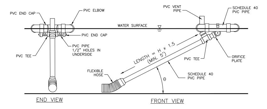
SCHEMATIC OF SKIMMER TAKEN FROM PENNSYLVANIA EROSION AND SEDIMENT POLLUTION CONTROL MANUAL, MARCH 2000.
