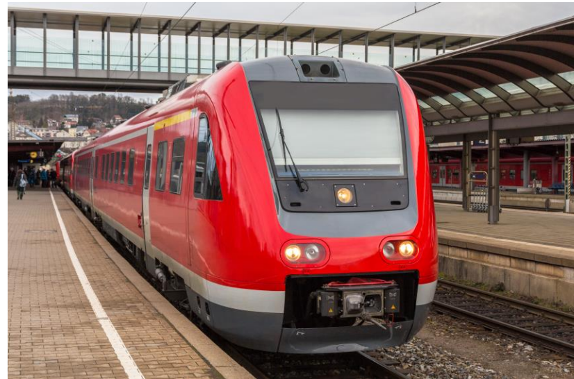
Multiple unit trainset each car has its own engine and can run independently or connected
