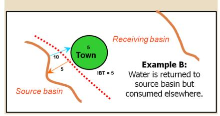
The amount of a transfer is determined by the amount of water moved from the source basin to the receiving basin, less the amount of water returned to the source basin and consumptive use in the source basin.
