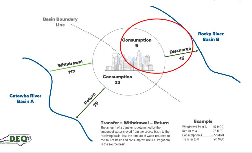
An IBT is a withdrawal, diversion or pumping of water from one source river basin to another river basin. The water from the source basin is treated and distributed to customers for everyday water usage, then collected and treated at wastewater treatment plants before portions are discharged to the receiving basin, resulting in the interbasin transfer.
