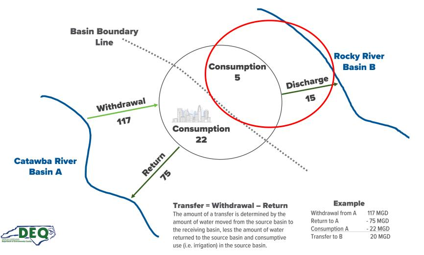
An IBT is avithdrawal, diversionor pumping of waterfrom one source rivebasin to another riverbasin. The water from the source basin isreated anddistributed to customers for everyday water usage,then collected and treated at wastewatertreatment plantsbefore portions are discharged to the receiving basin, resulting in the interbasintransfer.
