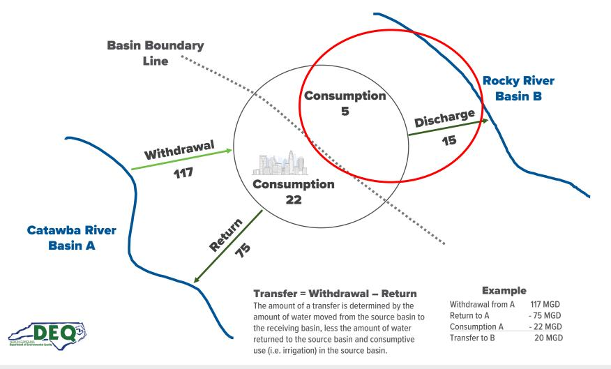
An IBT is avithdrawal, diversionor pumping of waterfrom one source riverbasin to another riverbasin. The water from the source basin isreated anddistributed to customers for everyday water usage,then collected andtreated at wastewatertreatment plantsbefore portions are discharged to the receiving basin, resulting in the interbasintransfer.
