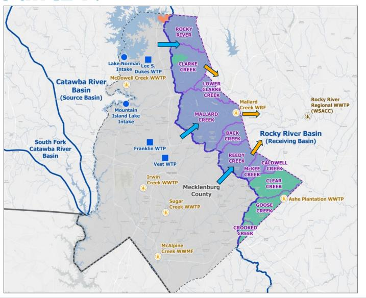
An IBT is a withdrawal, diversion or pumping of water from one source river basin to another river basin. The water from the source basin is treated and distributed to customers for everyday water usage, then collected and treated at wastewater treatment plants before portions are discharged to the receiving basin, resulting in the interbasintransfer.
