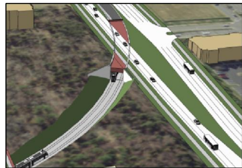
Underpass configuration example.
