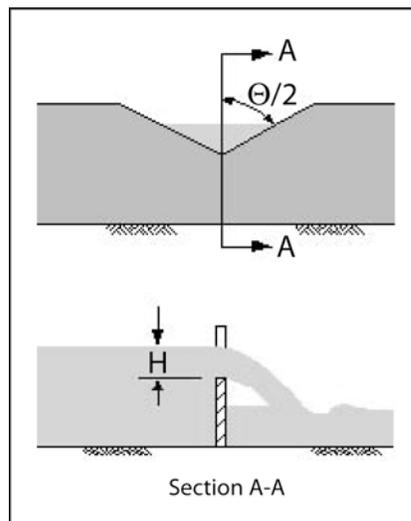
**Figure 6-5** V-Notch Weir
