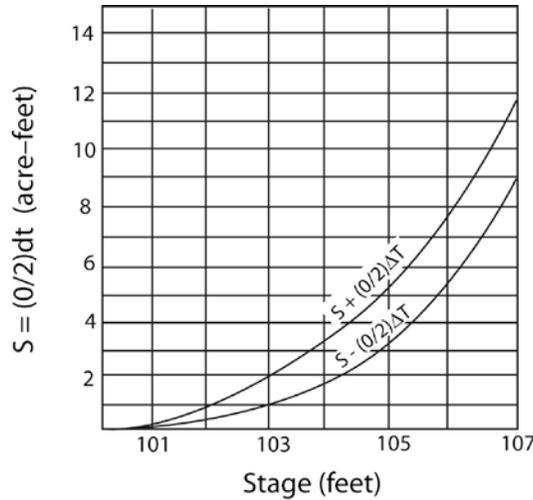
**Figure 6A-1** Storage Characteristics Curve
