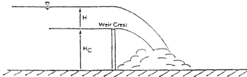
Figure 6-3 Sharp-Crested Weir
