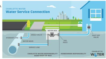
Service line is the pipe between water pipe under the street and meter box.
